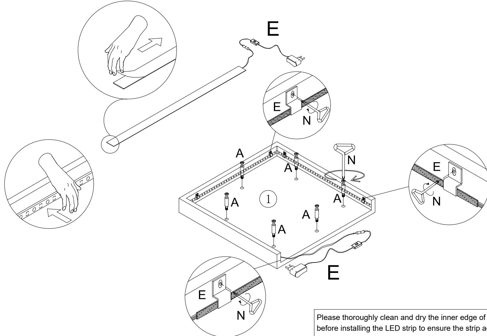
Please thoroughly clean and dry the inner edge of the panel before installing the LED strip to ensure the strip adheres securely.
